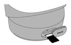
$\dot{\boldsymbol{\nabla}}$  Close tightly the waterproof cover after inserting the card.
