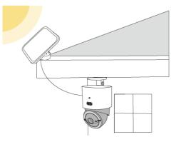
To absorb the most solar energy, choose the highly recommended orientation for installation based on your location.
