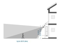
To ensure that no detection is missed, do not install the camera directly facing the monitoring area. Instead, maintain an angle to avoid any potential blind spots.
