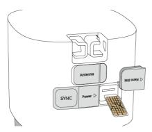
2. Rotate the camera and open the waterproof cover of the SD card slot, then insert a microSD card (not provided).
